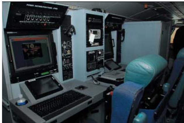
A Mission System Pallet aboard the HC-144A 2
